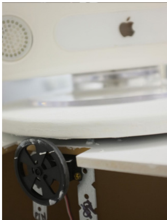
[ The motor and wheel used to drive the rotation of the lazy susan ]
